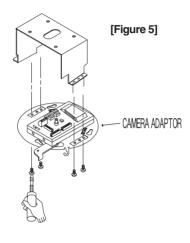
Pull the safety wire from the case body, and assembly it to the camera holder.
